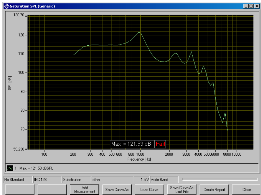
Fig. 33 Display window of saturation sound pressure level measurement
