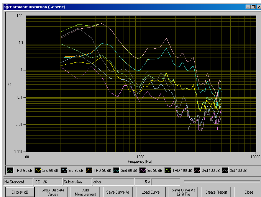
Fig. 34 Curve display of harmonic distortion measurement
