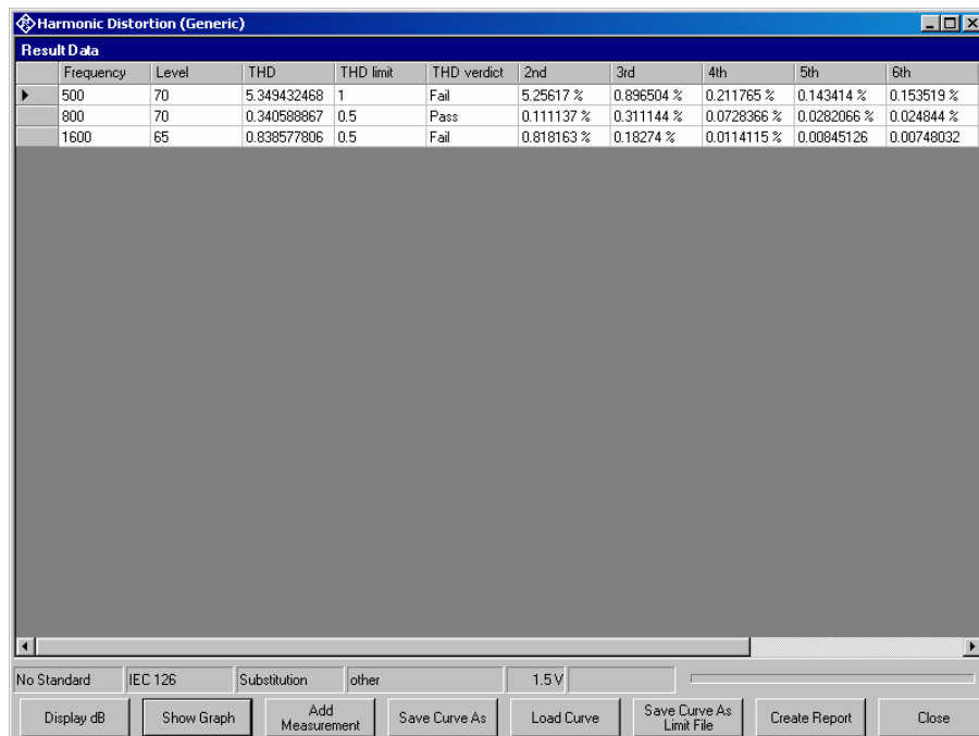
Fig. 35 Data table display of harmonic distortion measurement
