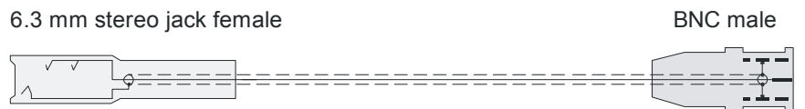
Fig. 3 Adapter cable to connect the R&S UPL-B7 battery supply cable to the "ANLG AUX OUT" of the R&S UPV
